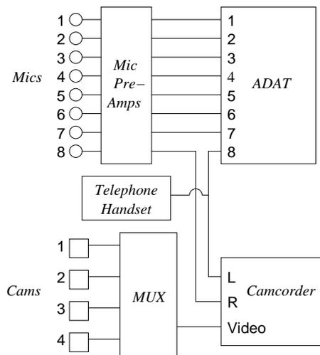
Figure 3: Equipment setup.
