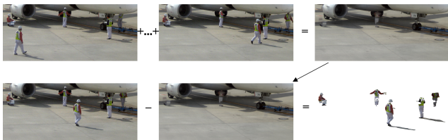
Fig. 1. Background subtraction. Top: averaging a sequence of images extracts their background. Bottom: subtracting that background from another image extracts its foreground.
